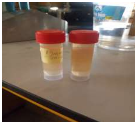
Image 2: Decolorized sugar using activated carbon
